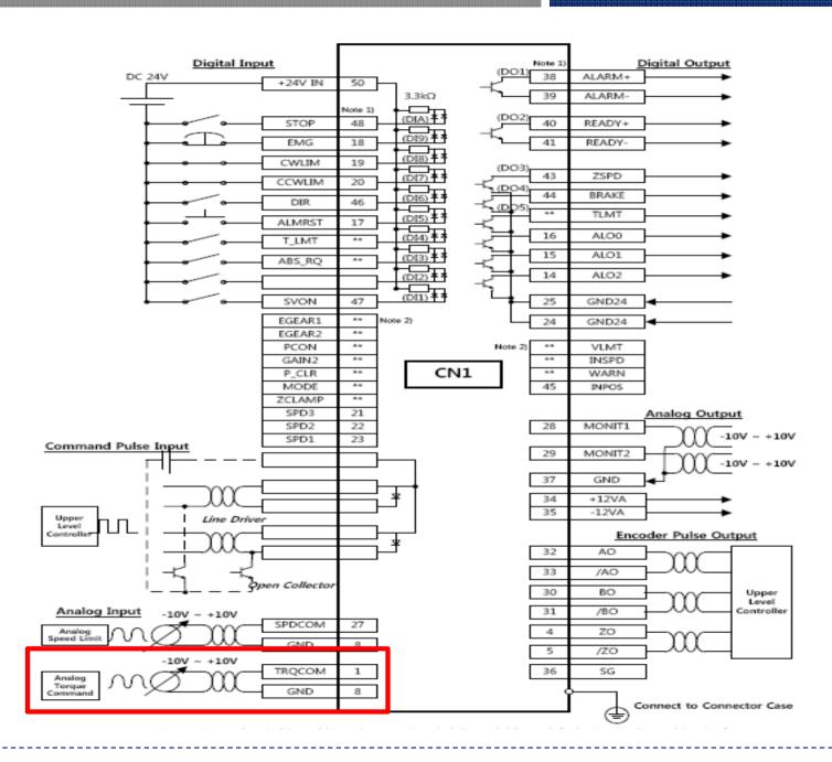
**Outline:** Torque mode is to use for controlling tension and pressure of machine.
