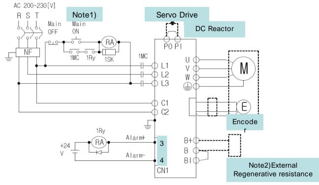
Note1) It takes approximately one to two seconds to output an alarm signal after turning on the main power(3Phase AC220V). Accordingly, press and hold the main power ON switch for at least two seconds.
